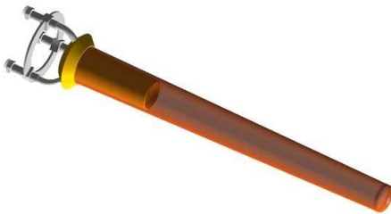
Figure 1.11: The 40 cm long cylindrical Kapton target cell used for g12 . Image source: [23].
